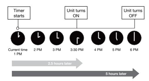
Example: If current time is 1:00PM, and the timer is set per the above steps, the unit will turn on 2.5h later (3:30PM) and turn off at 6:00PM.
