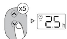
Point the remote at the unit and wait 1sec for TIMER ON to be activated.
