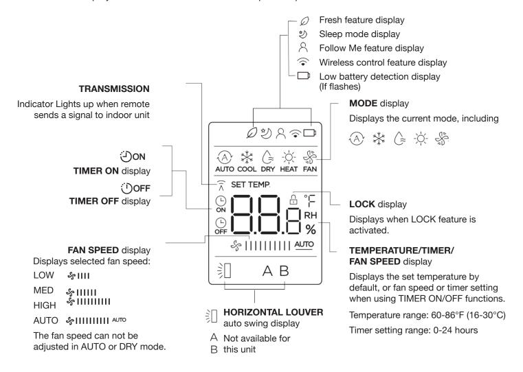
**NOTE:** All indicators shown in the figure are for illustration only. During the actual operation, only the relative function signs are shown on the display window.
