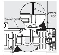
Connect the household water line to the water valve. Follow instructions in Connecting Ice Maker to Water Supply.
