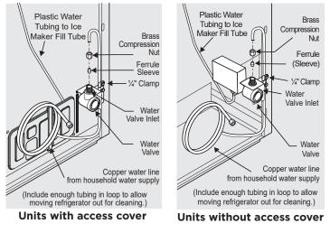
5. Secure the copper line to the clamp (as shown), using the existing screw.
