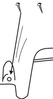
Figure 3. A pilot hole may need to be drilled to securely anchor the lag bolts. Make sure the lavatory is leveled before tightening these bolts. DO NOT OVER TIGHTEN, CHINA WILL BREAK.
