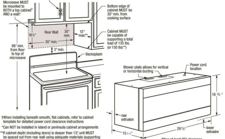
Locate 120V/60Hz grounded outlet inside upper cabinet
