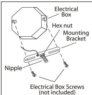
1. Attach nipple to mounting bracket. Adjust so it will clear hole in back of fixture and then lock nipple in place with hex nut. Mount the mounting bracket to electrical box using electrical box screws (not included).
