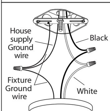
2. Connect the ground wires (bare copper or green) from your fixture to the ground wire (bare copper or green) or ground screw in the electrical box. Attach the black wire from the light fixture to the black wire in the electrical box. Attach the white wire from the light fixture to the white wire in the electrical box.
