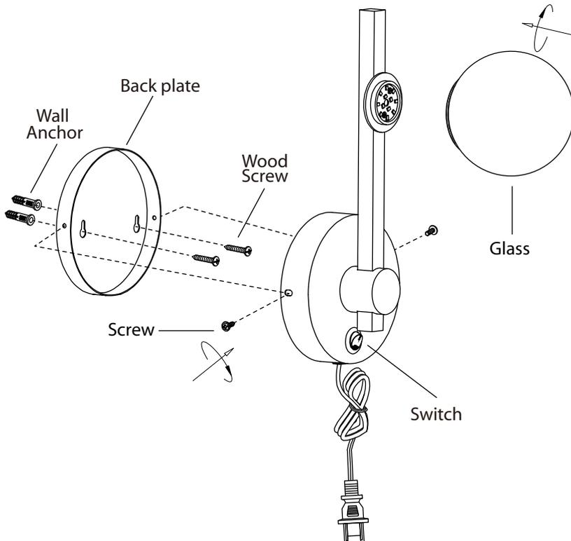
**1.** Remove the back plate from the fixture by unscrewing the 2 screws.
