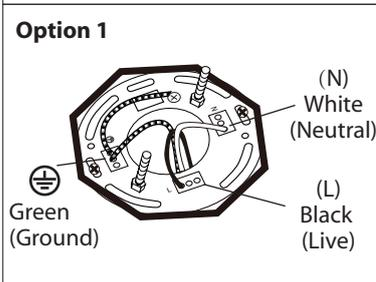
3. **Option 1:** Connect (push) electrical wires from electric box (house wiring) into correct inserts.
