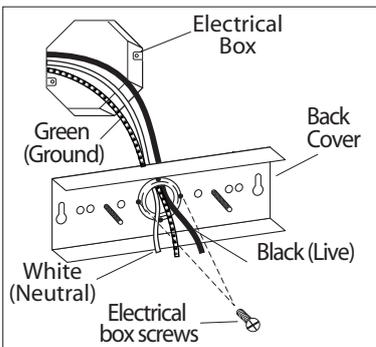
1. Feed power cords from the electrical box through the centre hole of the back cover. Align holes of back cover over electrical box and secure with electrical box screws (not included).
