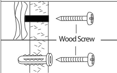
2. Additional support may be required for fixtures longer than 20". Position the fixture and add wood screws (one on each side) for the wooden studs or plastic wall anchor and wood screws for dry wall.
