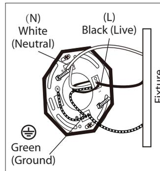
4. Connect (push) electrical wires from fixture into correct inserts.
