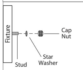
5. Tuck electrical wires into electrical box and position fixture over studs on mounting bracket assembly. Secure fixture in place with star washers and cap nuts.
