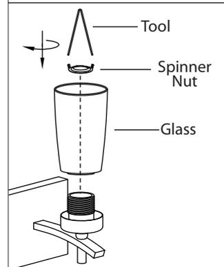
6. Remove spinner nut from socket. Position glass on lamp and secure with spinner nut.
