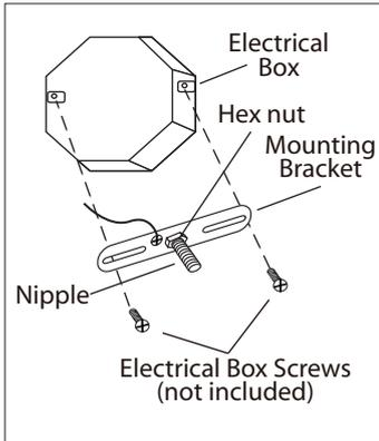
**1.** Attach nipple to mounting bracket. Adjust so it will clear hole in back of fixture and then lock nipple in place with hex nut. Attach mounting bracket to electrical box with electrical box screws (not included).
