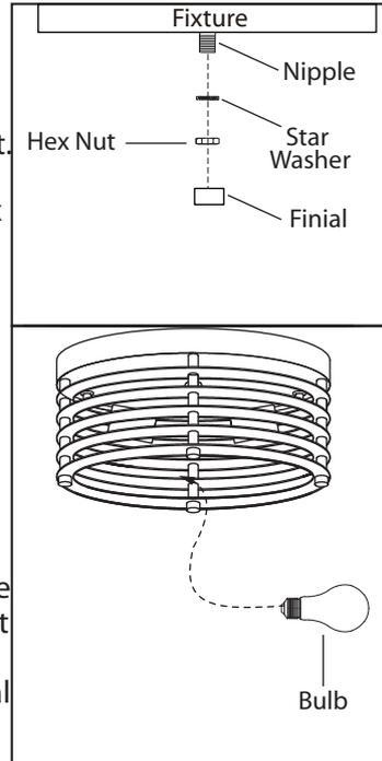
**4.** Secure the fixture to the nipple tightening by star washer and hex nut. Screw the finial to the nipple.
