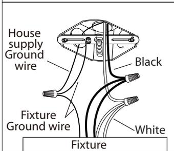
**2.** Connect the ground wires (bare copper or green) from your fixture to the ground wire (bare copper or green) or ground screw in the electrical box. Connect the black wires from the fixture to the black wire in the electrical box and connect the white wires from the fixture to the white wire in the electrical box.
