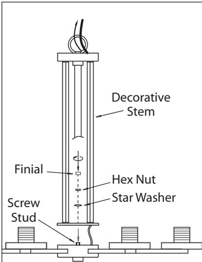
1. Slightly insert the decorative stem into the screw stud and tighten by a star washer, hex nut and the finial.
