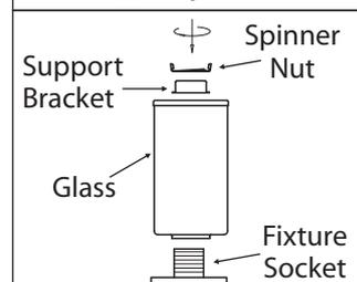
7. Remove spinner nut and support bracket from socket. Position glass on lamp and secure with spinner nut and support bracket.
