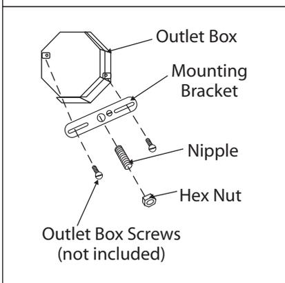
2. Attach the mounting bracket to the outlet box using electrical box screws (not included). Attach the nipple to the mounting bracket and adjust until it will clear the canopy when assembled (Place the canopy over the nipple and tighten the upper connector onto the nipple until snug. The upper connector should hold the canopy snug to the ceiling). Lock the nipple in the correct position using the hex nut.
