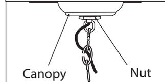
6. Once connections of wires are completed, carefully tuck wires and wire nuts into the outlet box making sure no bare wire (on the black and white) is visible at the wire nuts. Slide canopy into position and tighten in place by nut into position.
