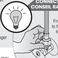
Firmly hand tighten the hose to the valve and add a quarter-turn using the proper wrench. Tighten more if needed.
