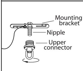
2. Determine the height that you would like to hang your fixture. Trim the cord and chain. Allow 10" of extra wiring for the electrical box connections.
