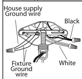
6. Connect the ground wires (bare copper or green) from your fixture to the ground wire (bare copper or green) or ground screw in the electrical box. Connect the black wire (or wire marked "SPT-1") from the fixture to the black wire in the electrical box and connect the white wire (or the wire with ribbed side) from the fixture to the white wire in the electrical box.
