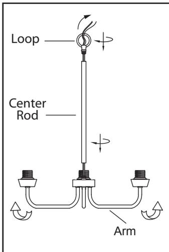
1. Spread the arms evenly. Screw the center rod to the fixture. Tighten the loop to the center rod.
