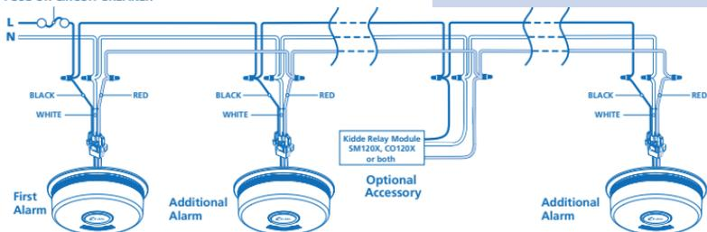
Figure 10-A, Interconnect Wiring Diagram
