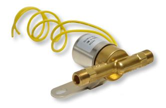
The Ranco<sup>®</sup> 4040 Series Solenoid Valve controls water flow to the humidifier to ensure proper humidity is delivered creating a more comfortable living environment. The 4040-001 solenoid valve has a strainer screen to filter out contaminants and eliminate build up in the humidifier. The 4040-001 kit includes an inlet compression fitting and ferrule to make installation simple.
