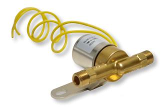
The Ranco<sup>®</sup> 4040 Series Solenoid Valve controls water flow to the humidifier to ensure proper humidity is delivered creating a more comfortable living environment. The 4040-001 solenoid valve has a strainer screen to filter out contaminants and eliminate build up in the humidifier. The 4040-001 kit includes an inlet compression fitting and ferrule to make installation simple.
