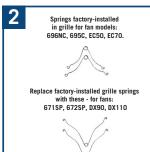
Attach new grille to fan with one grille spirng. Plug motor into pass-thru plug. Plus pass-thru into fan receptacle.
