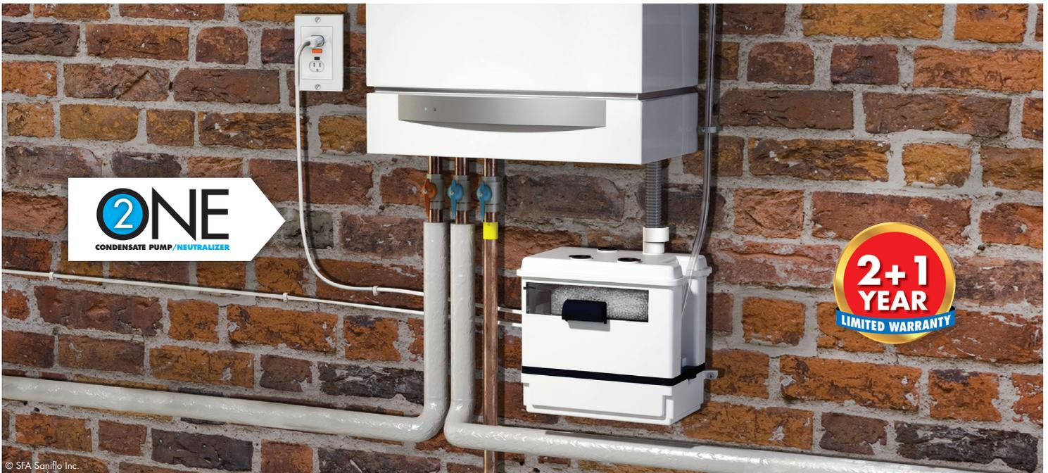
The Sanicondens Best is a pump used to **neutralize and pump condensate from condensing boilers, HVAC systems, water heater systems, etc.** The Sanicondens Best will pump condensate waste up to **15 feet in height and/or 150 feet away** from a soil stack.
