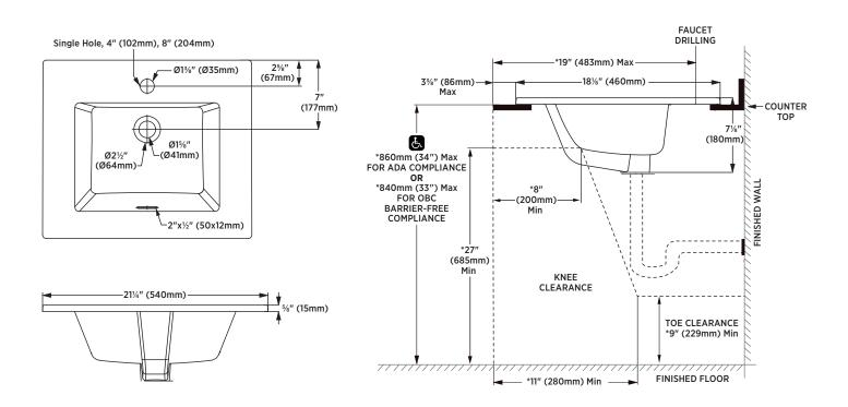
▲ NOTE: Starred measurements comply with ADA and OBC barrier free accessibility requirements.
