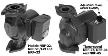
**Great for home heating applications**: Choose from five different models, including the new 3-speed models, NRF-25, -36 & -45. Except for the NRF-45, all models share the same "A" dimension as the famous series 100 pumps. Rated to 150 psi at 225° F. System (water) lubricated.
