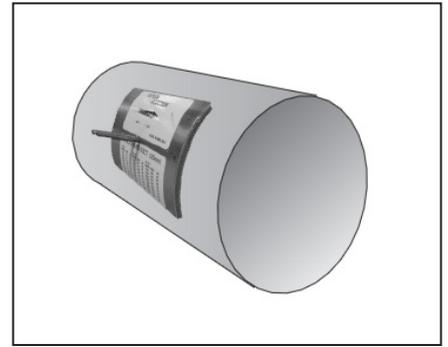
**1** Cut hole in duct and insert flow measuring station. Make sure that the flow measuring station's air direction arrow points in the direction of the airflow. Secure the flow measuring station with duct tape.
