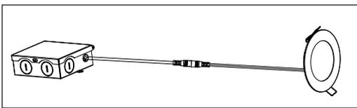
Hole Cut Size - Round 4":  $\varnothing 4 \frac{1}{4}"$  (108 mm)
