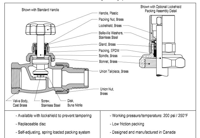
Dahl tailpiece wrench must be used to install union tailpiece
