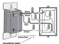
This wire is used in 3-way installations only. For single pole installations, do not remove insulating label.
