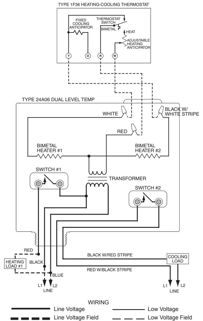
**Fig. 3. Using Heating-Cooling Thermostat to Operate Heating and Cooling Loads**
