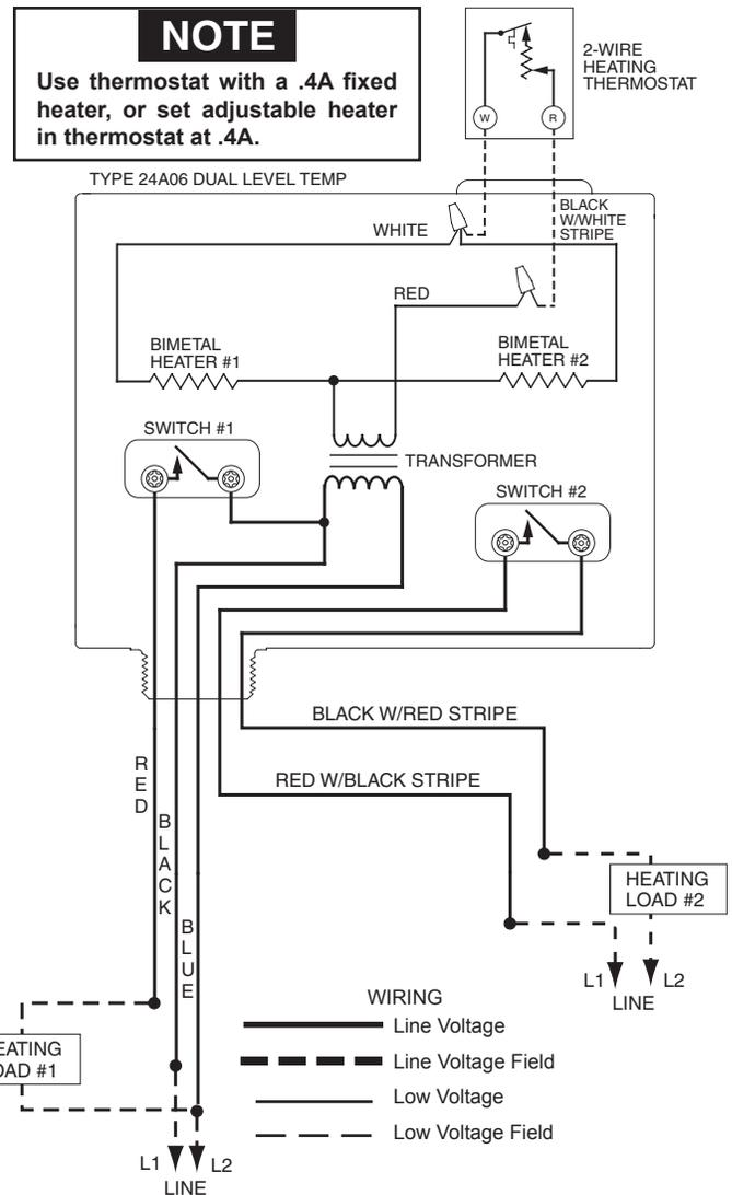
Fig. 2. Using Two-wire Heating Thermostat to Operate Two Separate Heating Loads
