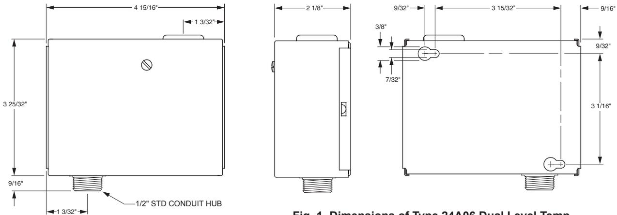
Fig. 1. Dimensions of Type 24A06 Dual Level Temp
