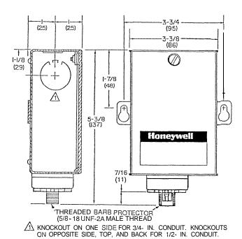
Fig. 1. P658A Switch Approximate Mounting Dimensions in Inches (Millimeters).
