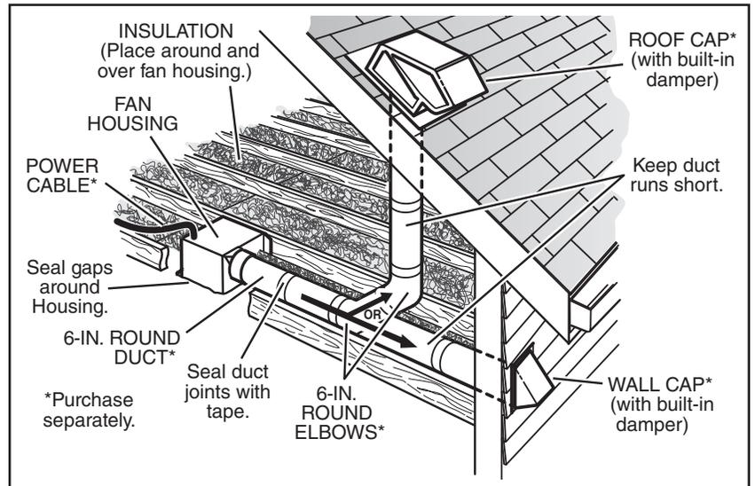
The ducting from this fan to the outside of the building has a strong effect on the air flow, noise and energy use of the fan. Use the shortest, straightest duct routing possible for best performance, and avoid installing the fan with smaller ducts than recommended. Insulation around the ducts can reduce energy loss and inhibit mold growth. Fans installed with existing ducts may not achieve their rated airflow.
