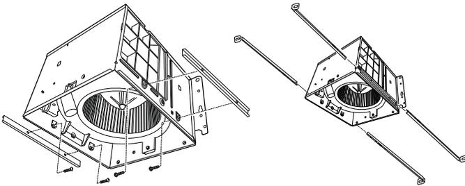
Sliding hanger bars are provided to allow for accurate positioning of housing anywhere between framing. They can be used on all types of framing (I-joist, standard joist, and truss construction) and span up to 24".
