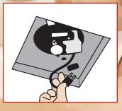
3 Install new motor assembly into existing fan housing.
