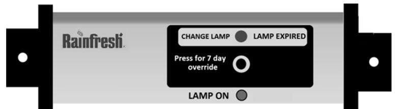
**UV Power Source Initialization Sequence:** When AC power is applied to the UV ballast, the lamp is ignited as indicated by the green lamp-ON LED and alarm buzzer consisting of three buzzer beeps and three red timer LED flashes.
