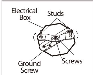
**2.** Position mounting bracket so that the fixture will sit level once it is mounted to the wall. Tighten screws to hold in place.
