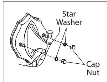
**4.** Once connections of wires are completed, carefully tuck wires and wire nuts into the electrical box making sure no bare wire is visible at the wire nuts. Install the light fixture to the wall by aligning the hole(s) in the fixture with the studs on the mounting bracket. Secure in place with cap nuts and star washers.
