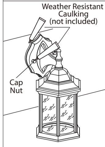
**5.** After installation, seal around the top and side perimeter between the fixture and the wall surface with weather resistant caulking. The bottom should be left un-caulked to prevent moisture build-up. Apply a small amount of weather resistant caulking around the side perimeter between the cap nut and mounting plate.
