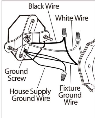
**3.** Firmly attach the fixture ground wire (bare copper) to the mounting bracket with the ground screw (by wrapping around the ground screw) and then connect it to the house supply ground wire with a wire nut. Connect the black wire from the fixture to the black wire in the electrical box and connect the white wire from the fixture to the white wire in the electrical box.
