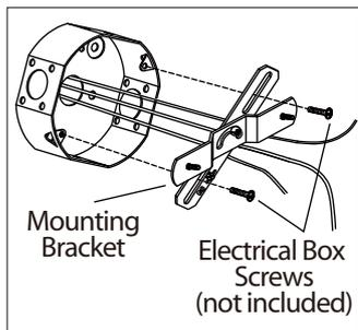
**1.** Mount the mounting bracket to electrical box using electrical box screws. Make sure the studs on the mounting bracket are facing out from the electrical box.
