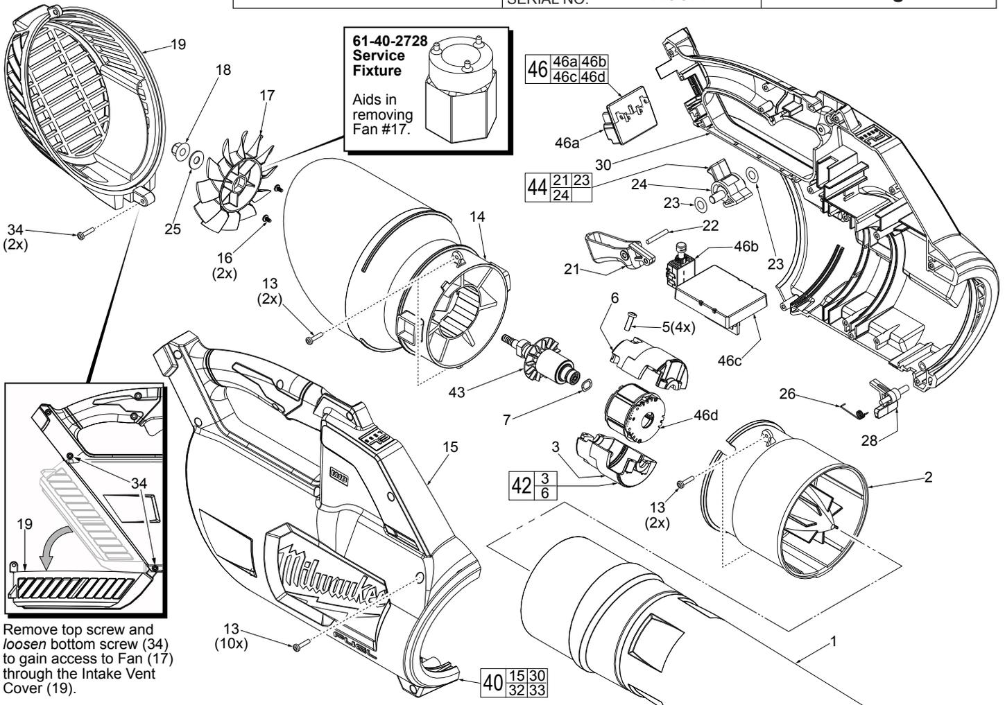
Remove top screw and loosen bottom screw (34) to gain access to Fan (17) through the Intake Vent Cover (19).
