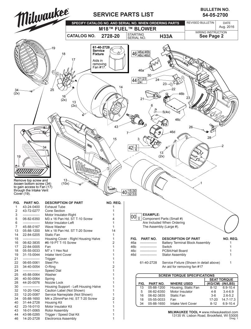
A Speed Dial with O-Rings (23) on each side 1 Trigger with Compression Spring (20) 46b On-Off Switch Abb On-Off Switch
