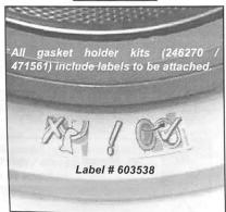
Attach advice label on gasket holder directly underneath door (at 6:00 position). Don't place label into spring clamp slot.
