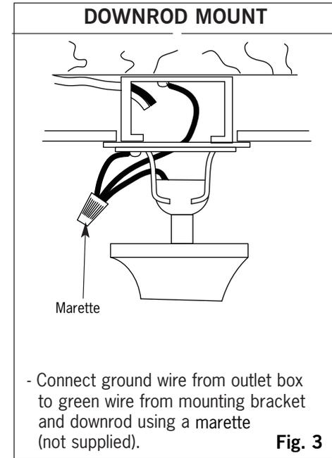
**NOTE:** Once ground wires are connected, carefully tuck wires and marette into the outlet box making sure that the wires are clear of the hemisphere and downrod when positioned in mounting bracket (Downrod Mount Only).
