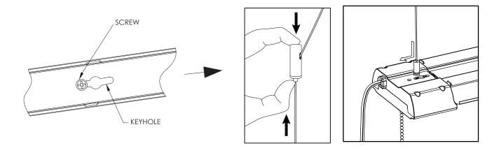
The **LSHOP series** is an integrated solution for quick and easy installation. Equipped with an keyhole, it is the fastest way to surface mount this workshop light. This is just as easy for suspended installation; with adjustable suspension cables included then just make the electrical connection. No need to remove the lens or open the luminaire.
