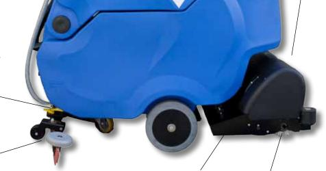
Integrated hopper to collect small solid debris.
