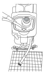
Check that the suction filter is undamaged and clean
