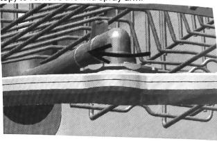
Reverse the procedure to install the spray arm.
