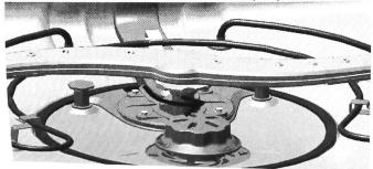
New Lower spray arm has the metal shields on the bottom. Reverse the procedure to install the spray arm. Make sure the spray jets are pointed upwards.
