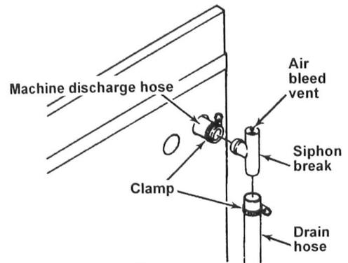
For machines with top drain hose connector located in upper left:
