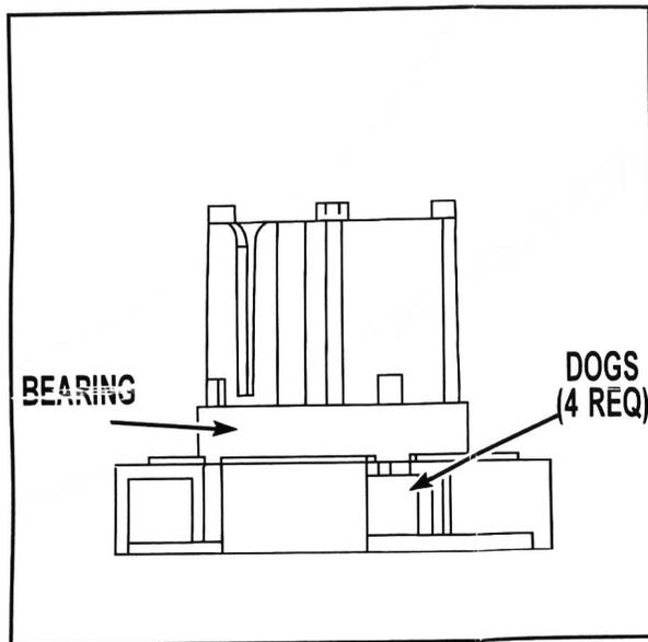
A. Assemble four (4) dogs into slots of agitator cam as shown in Illus. A.
