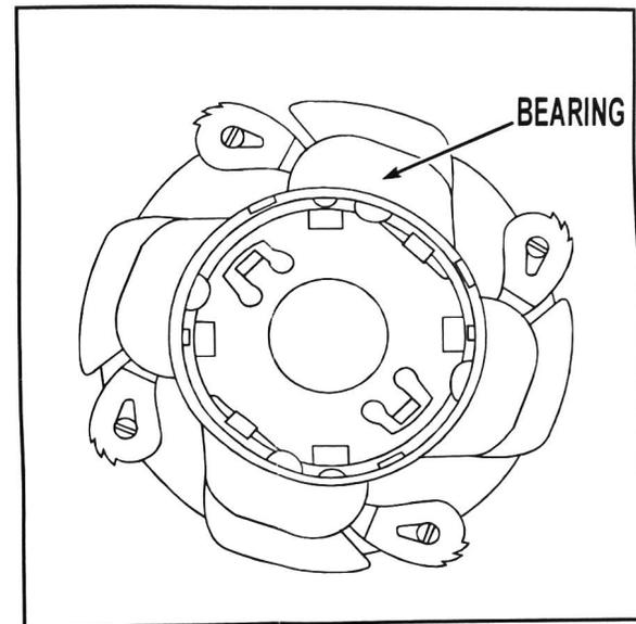
B. Bearing should be oriented and pushed all the way down to lock dogs in place, as shown in Illus. B.
