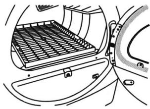
If the drying rack does not fit correctly in your Dryer, follow the steps below to move the support rod to the next hole.
