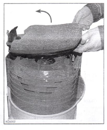
Using a long blade Phillips screwdriver, remove the 4 screws retaining the motor chamber to the unit.
