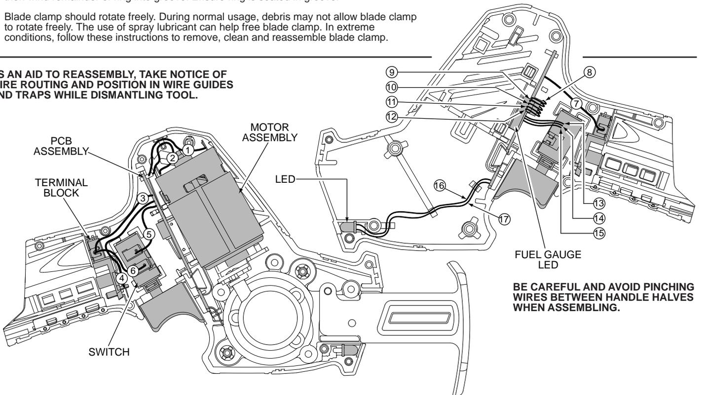
BE CAREFUL AND AVOID PINCHING WIRES BETWEEN HANDLE HALVES WHEN ASSEMBLING.
