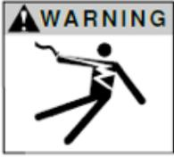
**⚠ WARNING** Disconnect power from all electrical equipment housed within the sump system before working on or around the sump pump or battery backup system beginning with 115 VAC powered pumps, level switches, and charger controllers; followed by DC powered items. Includes all items such as pumps, level control switches, Charger/Controller Unit, and battery systems.
