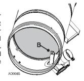
NOTE: Make sure the filter is installed so that the pull tab (A) is accessible A for future filter removal.
