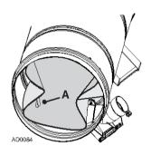
Squeeze the filter in order to move it past the inlet opening (B) Let the filter bear against the unit wall by releasing the pressure. Make sure to place the rigid ring in its groove to ensure proper sealing.
