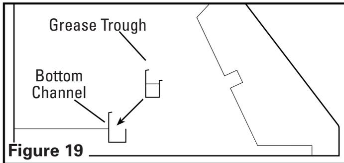
3. Install the baffle filters along with any spacer bars that are required by inserting the top of the filter into the top channel of the hood, then slide the bottom of the filter into the bottom channel. The filters have a top and a bottom. The bottom of the filter will have small drain holes. These holes must be facing down towards the grease trough to be effective. In models with spacers, it is easiest to install the spacer(s) first and the grease filters last (Figure 20).
