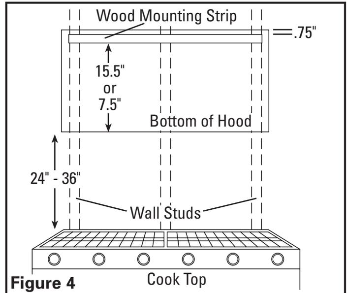
2. Attach the wood strip that was removed in **Section 1 Step 2** in place and confirm it is level. Secure in place using the provided 2" mounting screws making sure the screws are fastening into the wall studs (**Figure 5**).
