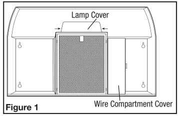
4. Install the included 26 watt GU24 fluorescent lamp into the lamp holder by lining up the pins on the lamp base to the socket of the lamp holder and turning the lamp body clockwise until the lamp snaps into place and is firmly seated in the lamp holder. Install a 4 watt maximum type C7 (candelabra base) night light (not included) into the side lamp holder and reinstall the lamp cover by squeezing the cover's sides and fitting them into the slots on the hood.
