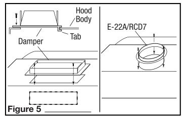
**NOTE**: If installing into existing construction and you will not have access to the ductwork once the hood is in place, make ducting connections at this point. Refer to the Ducting Section for instructions.
