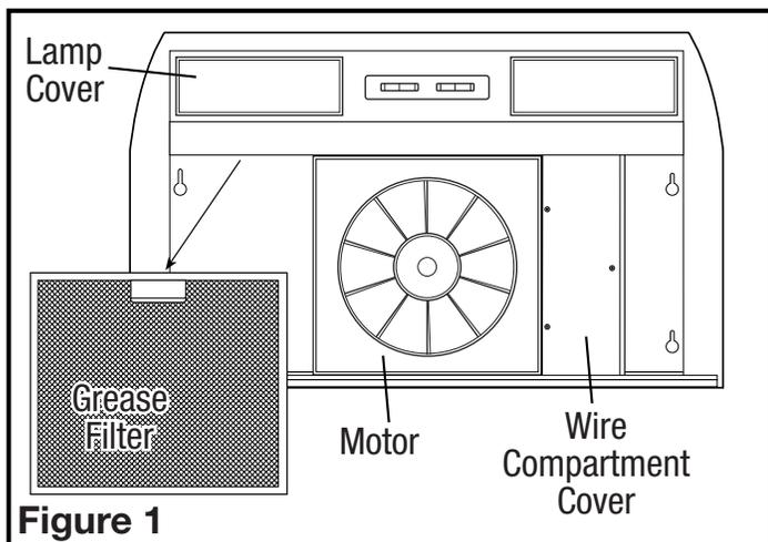
4. Install the included 18 watt GU24 fluorescent lamps into the lamp holder by lining up the pins on the lamp base to the socket of the lamp holder and turning the lamp body clockwise until the lamp snaps into place and is firmly seated in the lamp holder. Install a 4 watt maximum type C7 (candelabra base) night light (not included) into the side lamp holder and reinstall the lamp cover.
