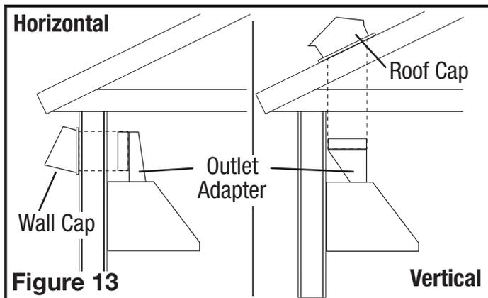
**NOTE:** When determining the outlet adapter to be used, make sure to consider the clearance within the cabinet space. Typically a horizontal Outlet Adapter will need to be used if you will be venting out to a wall cap.
