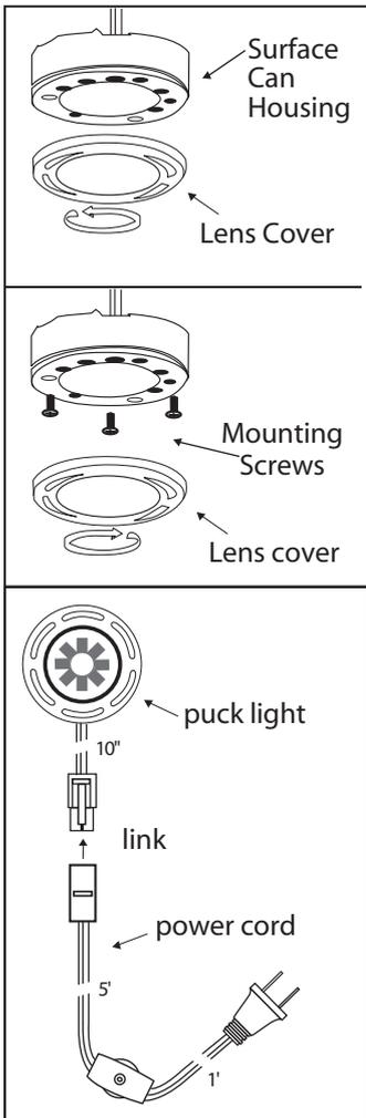
1. Remove lens cover by twisting counter-clockwise.
