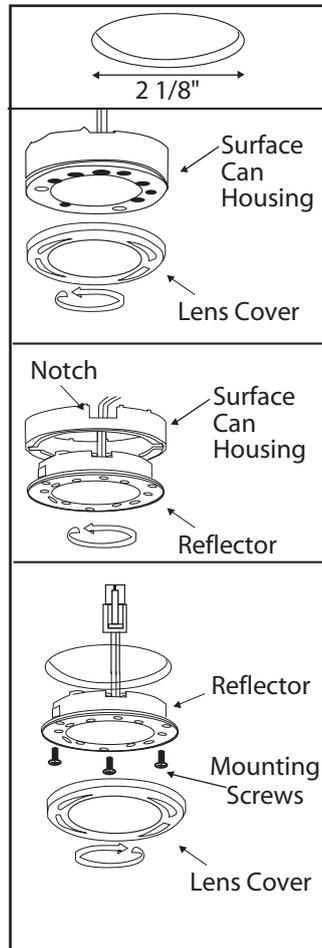
1. Drill a 2 1/8" hole in the underside of the cabinet
