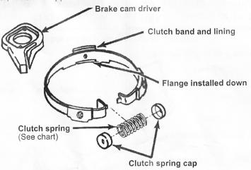
Clutch Band and Lining Assembly
