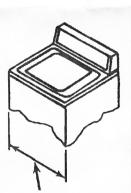
24" or 27" Regular, large capacity, Extra and Super capacity. Use 3946792 blue spring.
