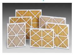
The MERV 11 pleated filters incorporate a 100% electrostatically charged synthetic media with an ASHRAE 52.2 MERV 11. The media is chemically bonded to a metal grid on the air-exiting side, preventing fluttering, and maintaining uniformity of the pleats. The filter pack is enclosed in a heavy-duty, moisture resistant, die-cut frame that will not warp, crack or distort under normal
