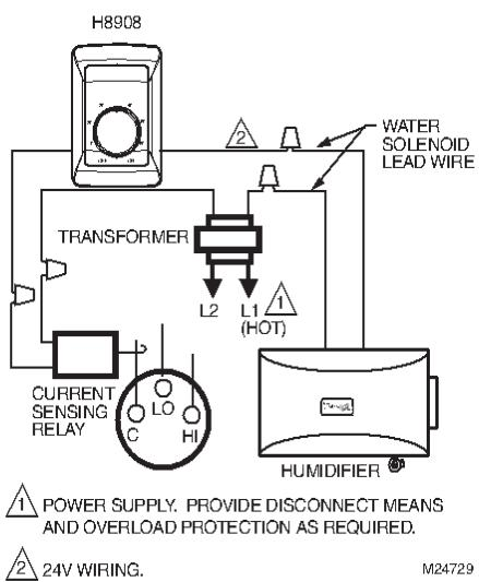
Fig. 14. Typical wiring diagram of current sensing relay with humidifier.
