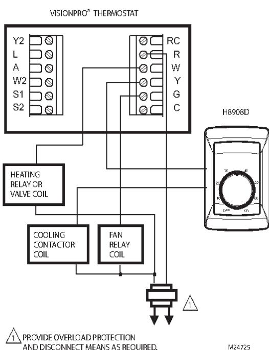
Fig. 18. Wiring H8908 with VisionPRO® Thermostat for dehumidification.
