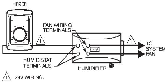
Fig. 16. Wiring H8908 with steam humidifiers.
