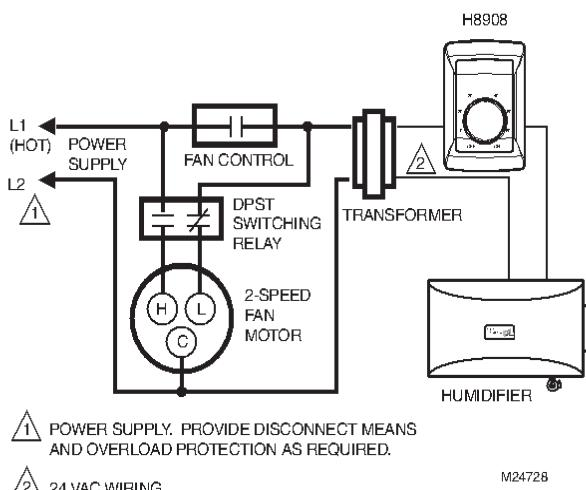
Fig. 13. Wiring H8908 with 2-speed fan motor.
