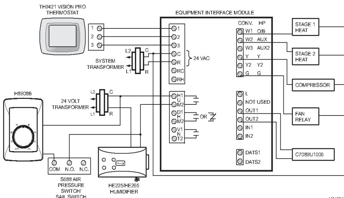
Fig. 17. Wiring H8908 with VisionPRO® IAQ on typical 2-stage furnace.
