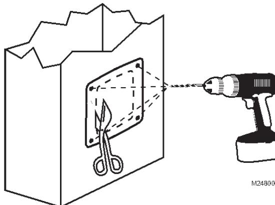
**Fig. 4. Drill and cut holes in duct.**
