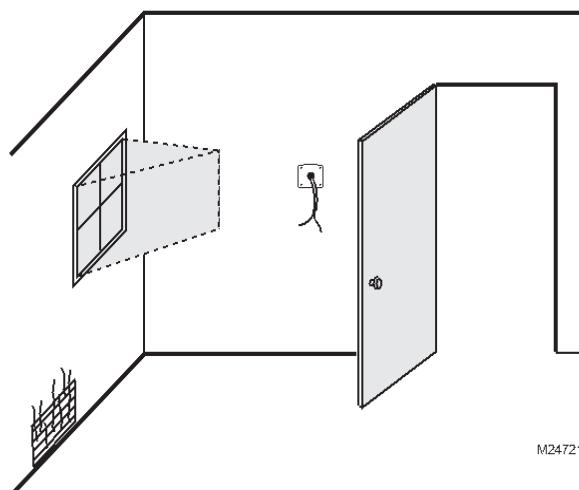
**Fig. 7. Run wire to the mounting location.**
