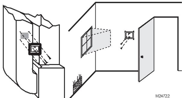
**Fig. 9. Mount base bracket to duct or remote location.**
