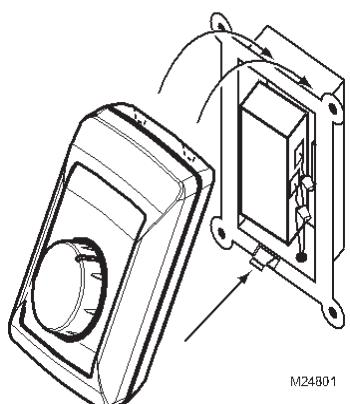
Fig. 11. Attach the humidistat to the base.
