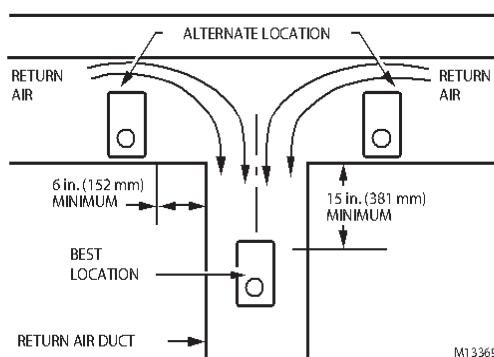
**Fig. 3. Duct installation locations.**
